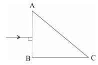
2. A suction device is arranged as shown in figure. The flow rate of air through the main pipe for which water suction will begin for the following data is Q.
